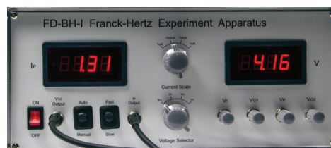
Franck-Hertz Control Unit with Internal FH Tube
