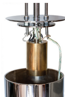
The sample heating assembly can be raised out of the oven on the telescoping support rod.
