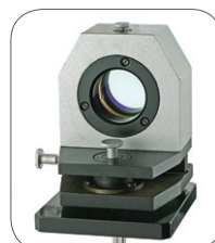
The étalon generates an interference pattern of concentric rings which is observed by a video camera.
