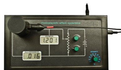
The main unit includes a voltmeter, nanoammeter, and light/voltage adjustment knobs.
