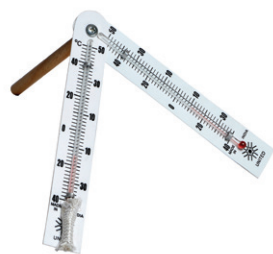
Assembled sling psychrometer includes wet and dry bulb thermometers.
